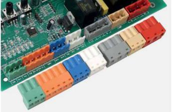
The advantage of the control board is the ease of barrier configuration. All terminals on the board are marked for easy connection. Easily removable terminals greatly simplify connection process.
