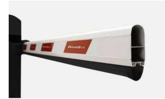
The boom is made of durable aluminium profile with 1.4 mm wall thickness, and reinforced inside with additional stiffeners. Boom profile has rounded edges providing high resistance to wind loads.
