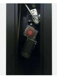
A special release mechanism allows you to lift and lower the boom manually, in case of power failure. The release system is located inside the body and is protected by a steel cover with a lock. The gear motor with release mechanism, the balancing mechanism, mechanical limit switches, and the control board are located inside the body.
